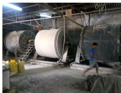
Existing ball mill
